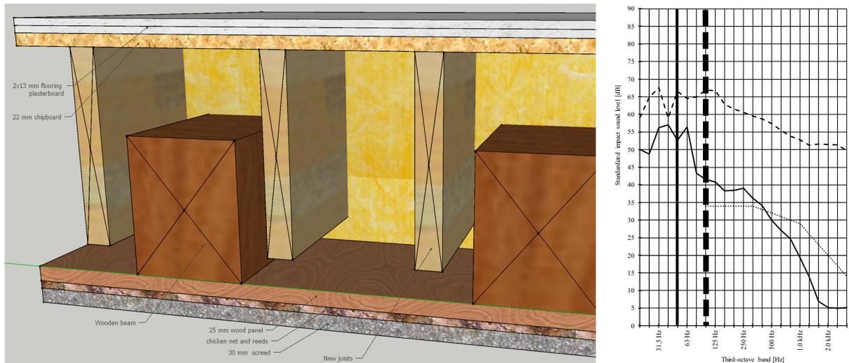
Figure 1. Exploded view of the rebuilt joists separating the attic from the apartment below. To the right is the impact sound insulation, before (dashed) and after (solid) the refurbishment. The dotted line is the reference curve after the change. The vertical solid line marks the 50 Hz limit of evaluation, the vertical dashed line marks the 100 Hz limit of evaluation.
