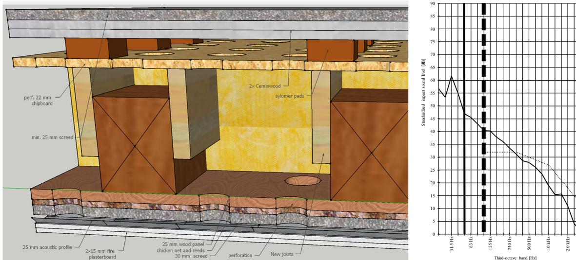
Figure 3. Exploded view of the separating construction. To the right is the impact sound insulation after the refurbishment. Dotted line is the reference curve. Vertical solid line marks 50 Hz limit of evaluation, the vertical dashed line marks 100 Hz limit of evaluation.
